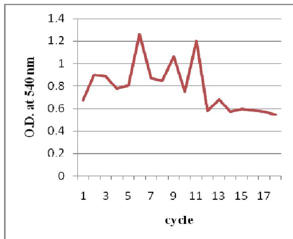
**Graph-3**chromium removal by continuous recycling through column
