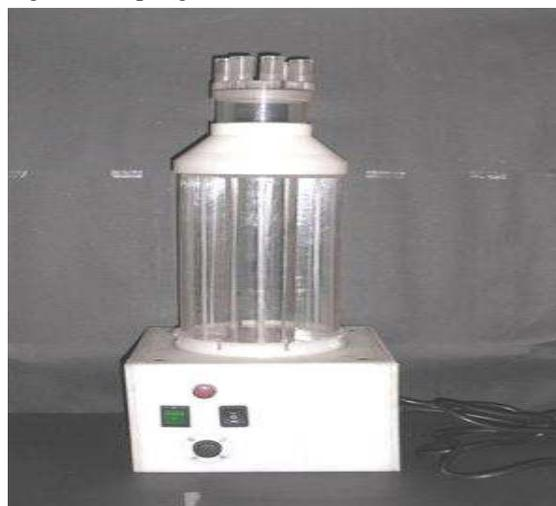
**Fig. 1b** Extended surface biofilm reactor (ESBR)
