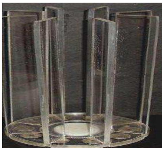
**Fig. 2** Inner configuration of the Extended surface biofilm reactor (ESBR)
