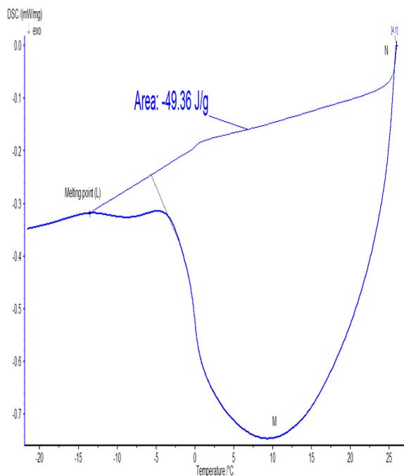
Figure 8 Melting point and latent heat of fusion
