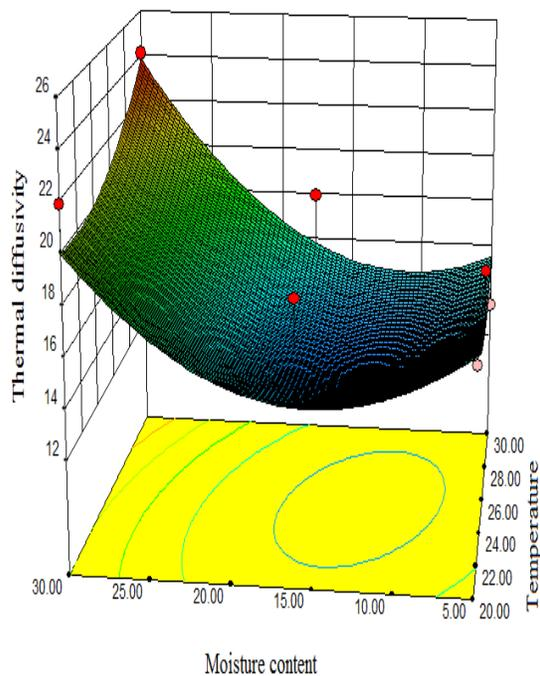
Figure 7 Variation in bulk thermal diffusivity with varying moisture content and temperature
