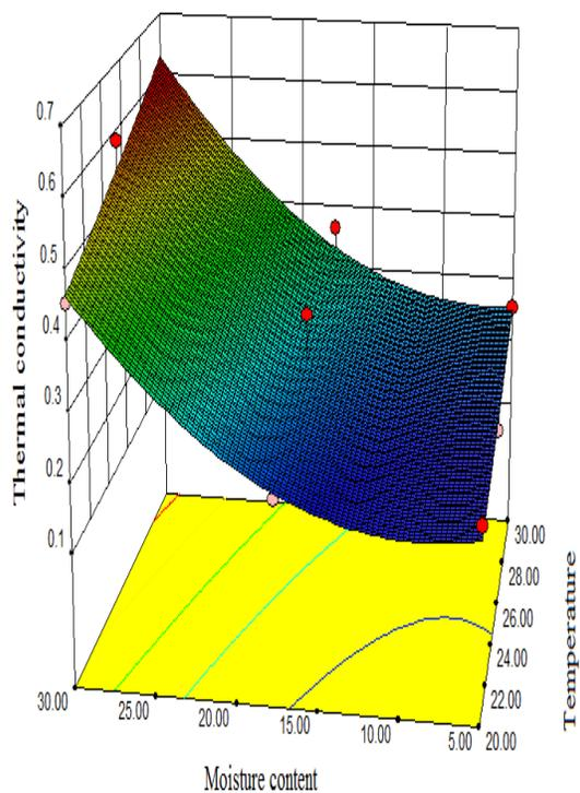
Figure 3 Variation in thermal conductivity with moisture content and temperature
