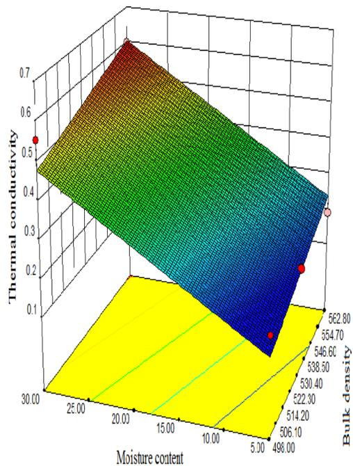
Figure 4 Effect of moisture content and bulk density on thermal conductivity of black pepper.
