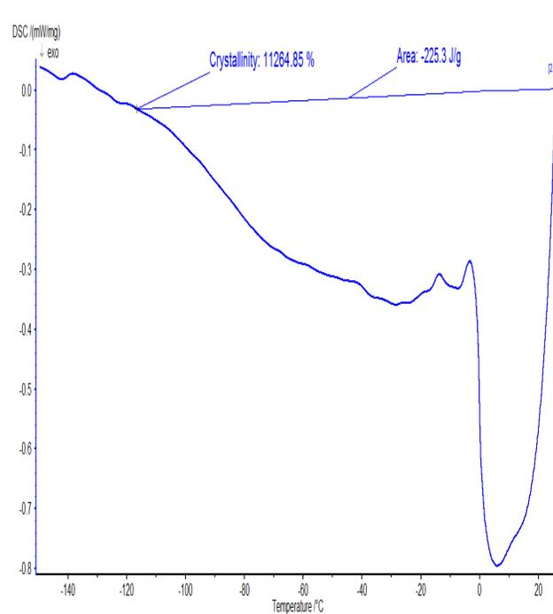
Figure 10 Heat of crystallization
