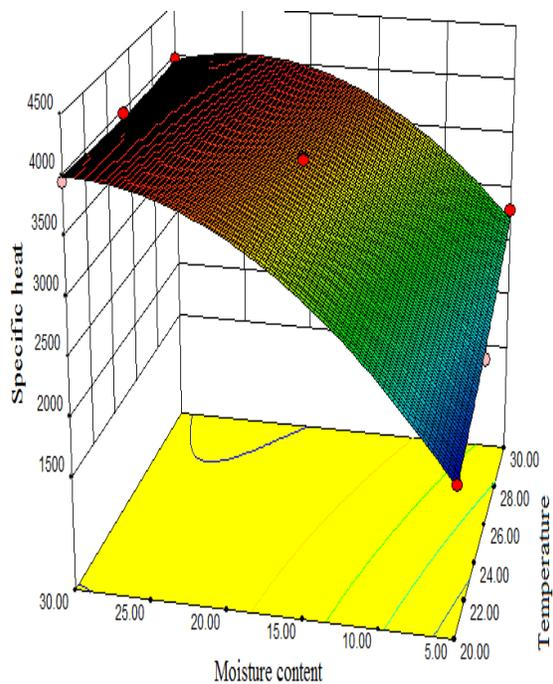
Figure 5 Variation in specific heat with varying temperature and moisture content
