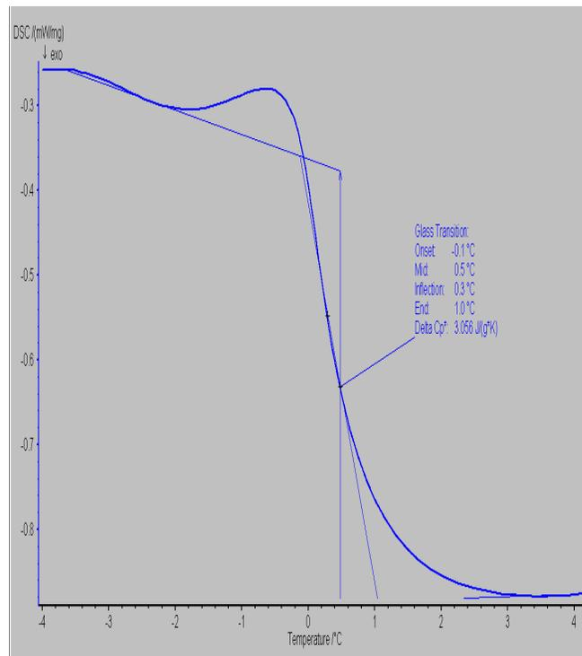
Figure 9 DSC thermograms showing the glass transition temperature of black pepper volatile oil
